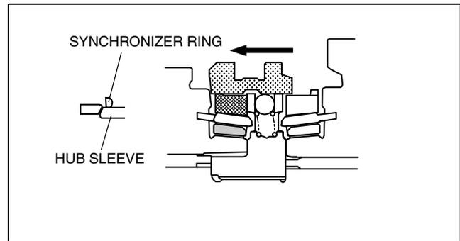
4. As the hub sleeve continues moving leftward, the hub sleeve then engages the synchro teeth to complete the shift.
