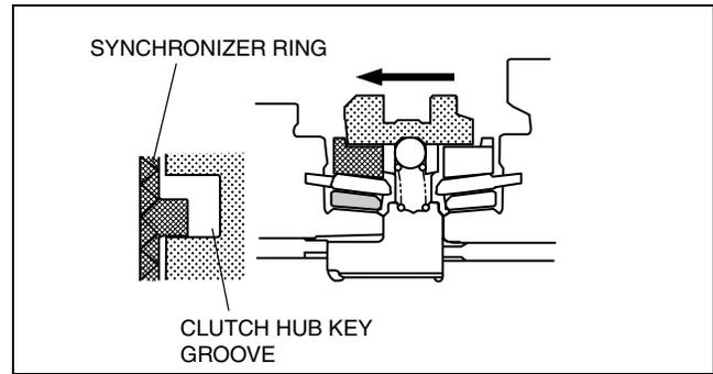
3. As the hub sleeve continues moving leftward, the difference between the rotational speeds of the second gear and the hub sleeve disappears, and synchronization is completed. When synchronization is completed, the hub sleeve rides over the ball and engages the synchronizer ring.
