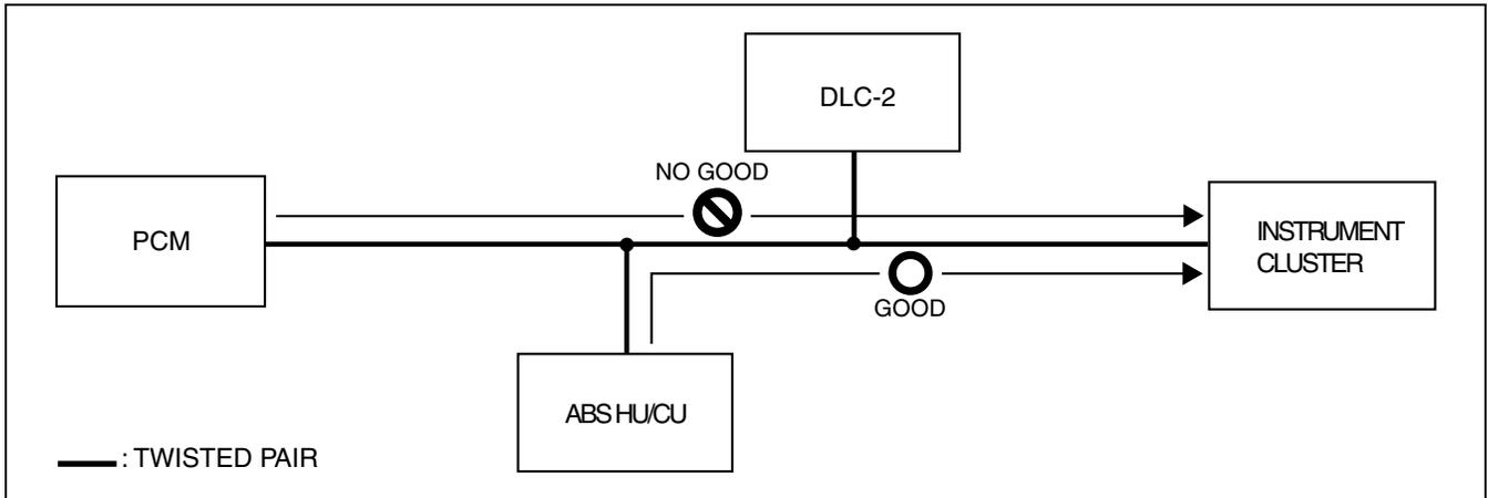
3. If there is a communication error between the ABS HU/CM and PCM, or between the instrument cluster and PCM, even if the communication between the ABS HU/CM and the instrument cluster is normal, it is probable that there is a malfunction in the PCM or PCM-related wiring harnesses.
